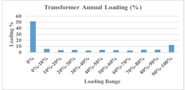
Solar inverter transformers operates in cyclic loading pattern in a 24 hour cycle. Also, their loading varies according to seasons & weather conditions. Loadings on solar inverter transformers are almost nil during night hours.
