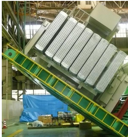
Figure 3 Inclination test of the transformer
