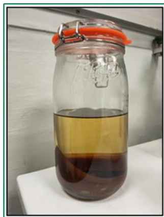
Figure 1: Glass vessel under vacuum containing oil, paper and copper
