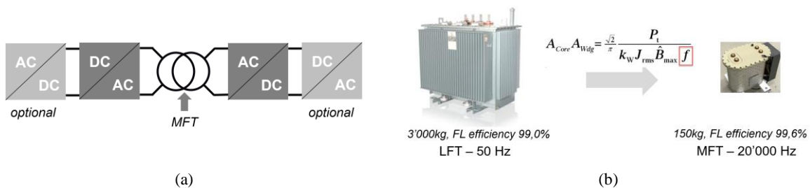
Fig. 1 – (a) Functional scheme of an SST cell. Several cells can be connected in series to reach MV. (b) Illustrative example of transformer frequency scaling, where MFT with same power and voltage rating features 95% weight reduction as compared to LFT.
