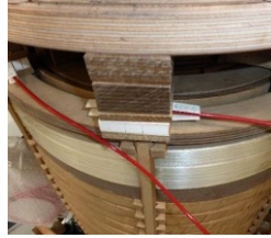
Figure 2: Built-in fibre-optic-clamping-pressure sensors at the winding top of a transformer
