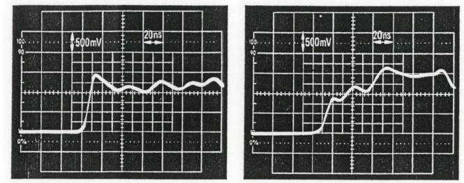
Considering this an upper frequency resolution of at least 5 Mhz is required. Looking at the winding diameter in large power transformers – which determines the length of a single turn – a frequency range of up to at least 10 Mhz can be reached.
