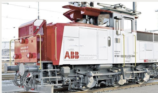
[2] ABB's 1ph, 1.2MW, 25kV 16,7Hz PETF (Source: www.abb.com )
