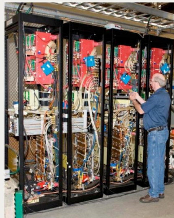
GE's 13.8kV to 465/ \sqrt{3} V, 60Hz, 1MVA SiC SST (Source: www.ge.com )
