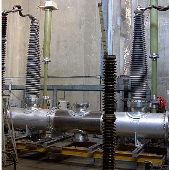
Figure 4: 420kV GIS circuit-breaker prototype using C4-FN-based gas mixture during breaking test in power laboratory
