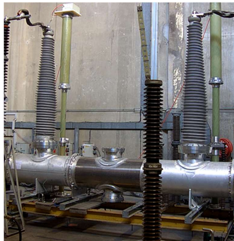
Figure 5: Full pole g 3 GIS 420 kV 63 kA synthetic testing in high power laboratories in CERDA, France
