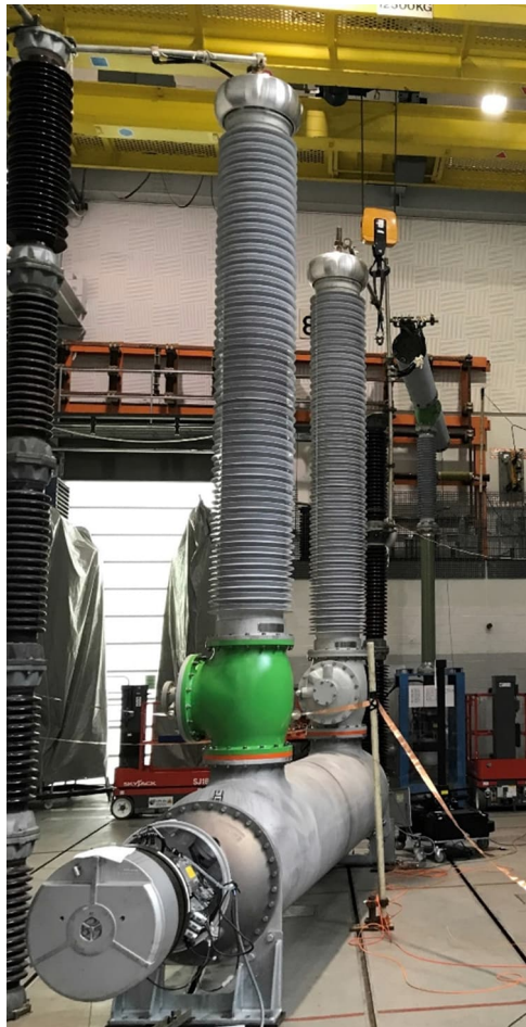
Figure 1. Double chamber 420 kV and 63 kA C4-FN-mixture-based circuit breaker.
