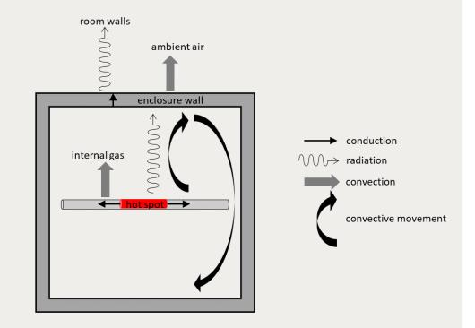
Convection is the only parameter that depends on the gas; all other parameters depend on the design
