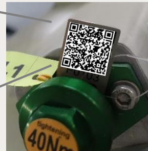
Gas inlet connection with gas ID
