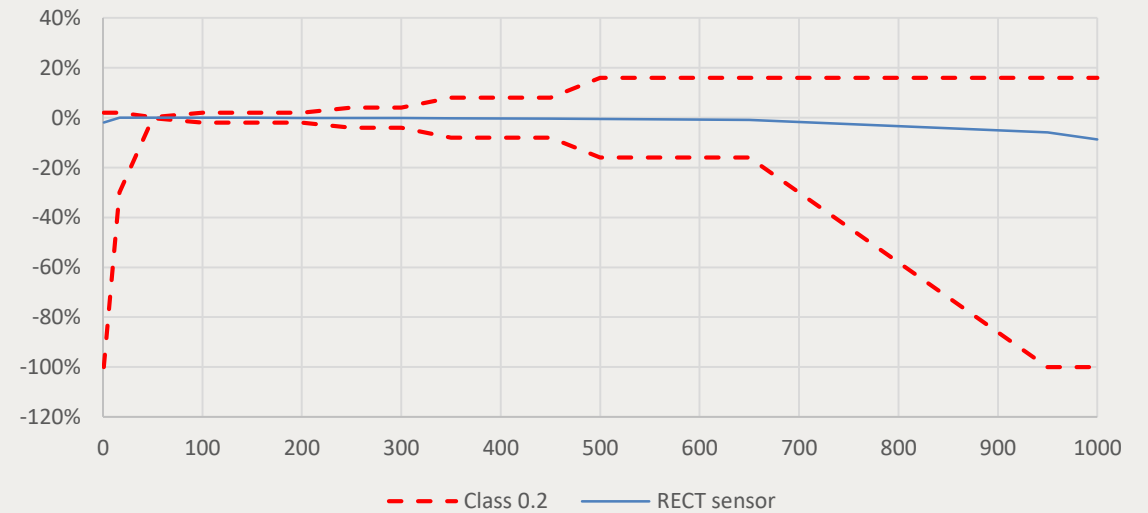
RECT Frequency response Measuring application CI 0.2S
