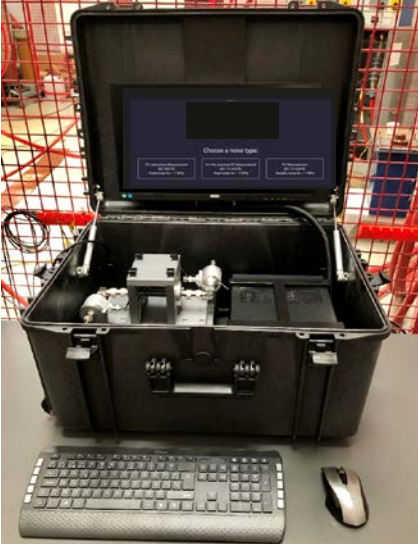
Figure 2. Testing Setup : PD emulator for PD analyser qualification
