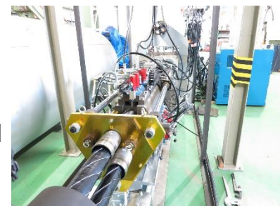
Fig 3. 3-phase simultaneous cable pulling machine
