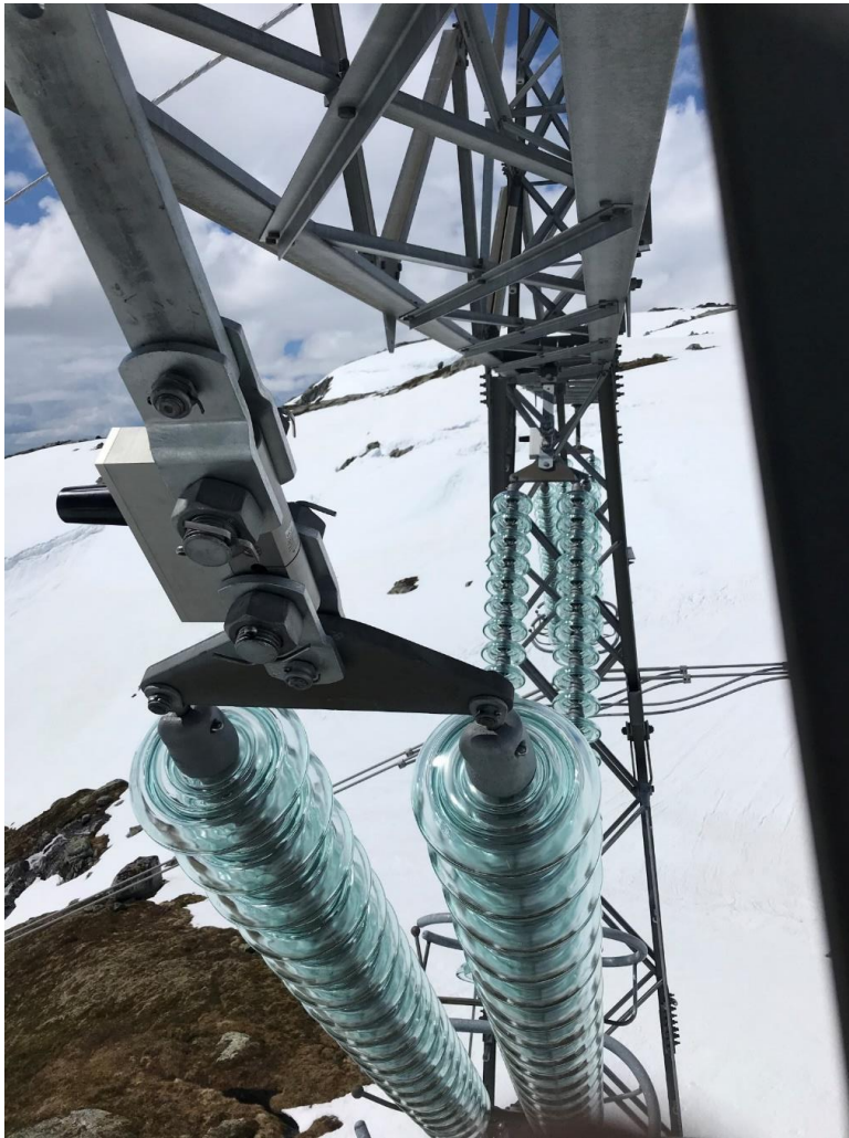
Figure 1: Tension load sensor (LoadTroll) developed by Kjeller Vindteknikk at Norconsult. Left shows an installation in the insulator string of a suspension tower.
