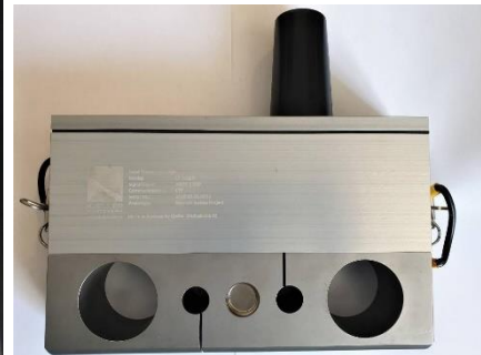
Figure 1: Tension load sensor (LoadTroll) developed by Kjeller Vindteknikk at Norconsult. Left shows an installation in the insulator string of a suspension tower.
