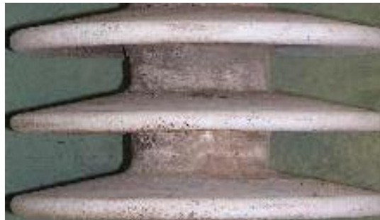
Fig. 1 Removed RTV long rod insulators for 5 years
