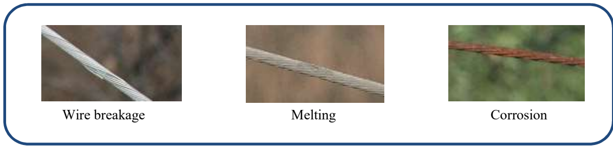
Fig. 2 Examples of failure state images used for learning
