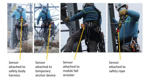
From the figure shown below, we can observe the other main objectives from the proposed wearable system: real time detection of misuse of PPEs or any other deviation from safety procedures and, consequently, alarm generation in real time to alert overhead line workers.
