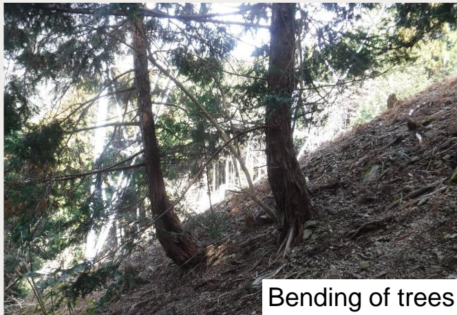
Fig.2 Example of landslide features in field survey
