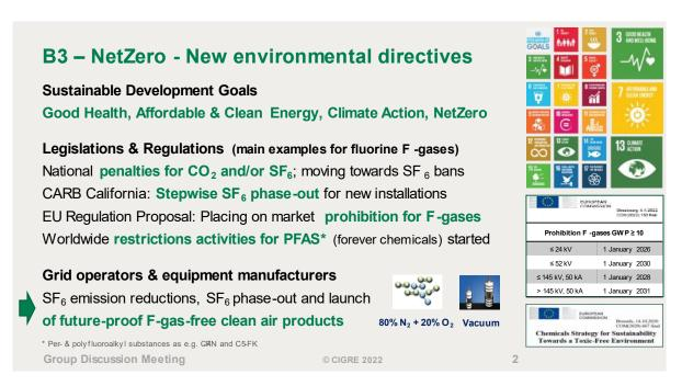
Slide 3 shows the status of introduction of zero  $CO_2$  emission T&D equipment, which can be only achieved with new equipment without any  $SF_6$  and with products using insulation gases based on clean air and vacuum interrupter switching technology with GWP = 0. More details can be found in e.g. [1, 2, 3, 4]
