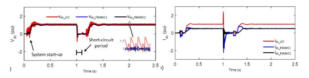
The Hybrid HVDC system was restored in 400 ms and it can be faster or slower depending on the system requirements.
