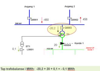
In addition, so is also the suggestion related to accuracy of the metering and station balance will be the new requirement. A maximum deviation for the whole metering balance to be 0,4% of the absolute loss/balance of the total absolute flow in the balance
