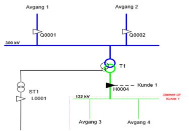
Metering station balance/loss in MWh: -480 + 458 + 20 + 0,1 = - 1,9 MWh
