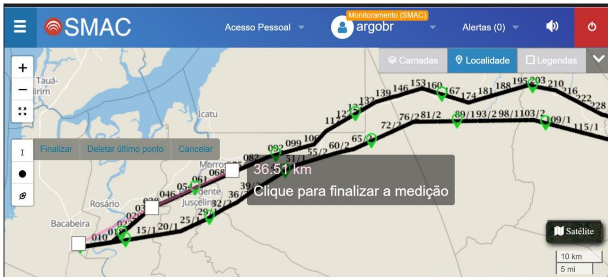
Figure 5 – Fault Distance Calculation and Transmission Tower Identification
