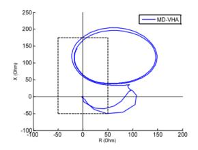
This OOS function has a non-conventional adjustment since it monitors quantities, not forming an electrical center. Also, this is a very sensitive function because its actuation leads to the split of two large power systems.
