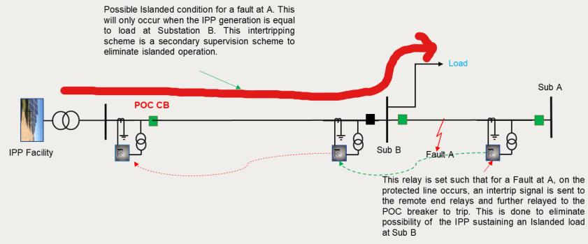
• During commissioning, the intercropping scheme is tested by verifying that the signal to disconnect is being received at the relevant point within the network.
