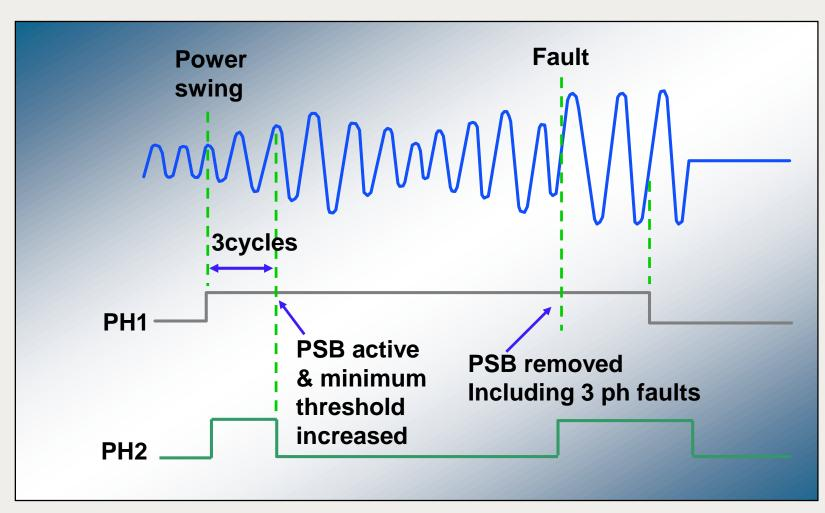
The trip time for any fault occurring during a power swing is exactly the same as had the swing not been present
