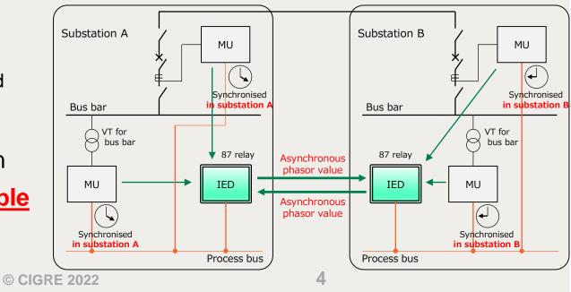
87 relay: Line current differential relay
