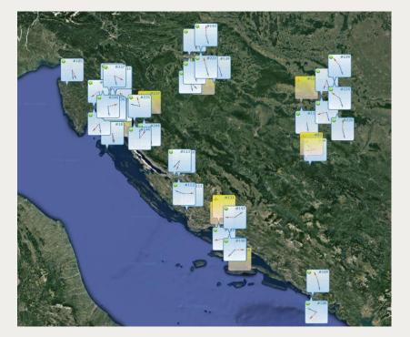
70+ PMUs: 400 kV: all lines 220 kV: all cross-border, almost all internal 110 kV: all cross-border, selected internal Selected generation units and WPPs Applications: integration with AGC controller, WAMS-based fault locator, synthetic inertial and primary frequency regulation response monitoring, ...
