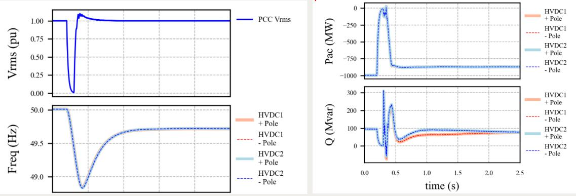
Lesson Learnt: It is very important to test multiple grid forming converters together to identify the possible interactions!
