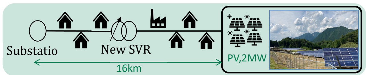
Fig 4. Commercial 6kV distribution system
