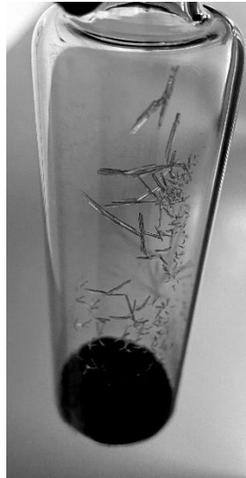
Figure 3. Two desiccants after thermal aging in C4-FN mixture
