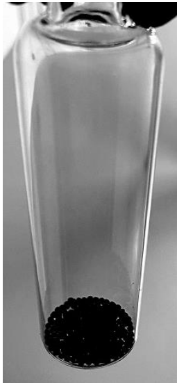
Figure 3. Two desiccants after thermal aging in C4-FN mixture
