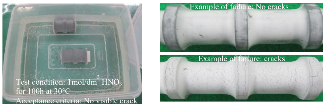
Fig.4 Nitric acid immersion test
