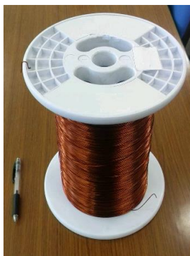
Figure 1: Enamel wire containing nanofiller (nanoclay) in the insulating layer
