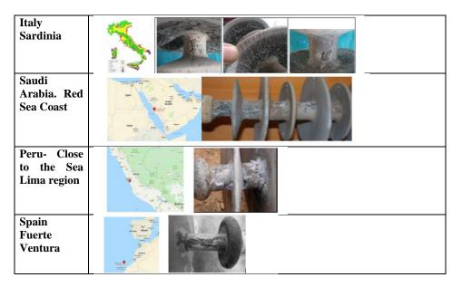
Figure 1 AC line insulators. Examples of degradations found in harsh environment [1].
