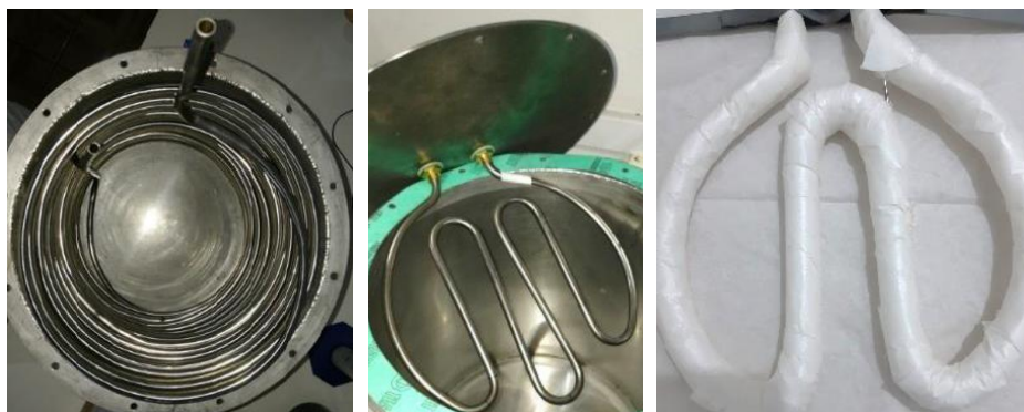
Fig. 3 – Test equipment developed for thermal fault modelling in liquid immersed system with aramid insulation: vessel with powerful water-cooling system + paper wrapped heating resistance
