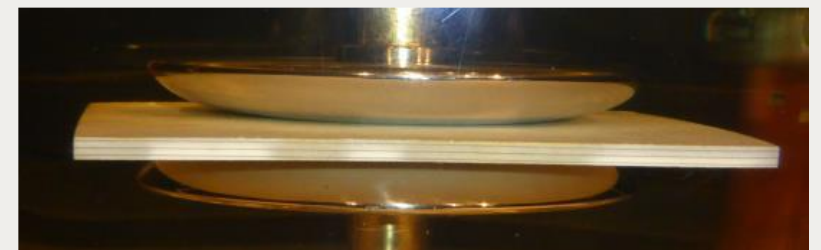
Example of laminated aramid board tested for PDIV at temperatures up to 120°C.
