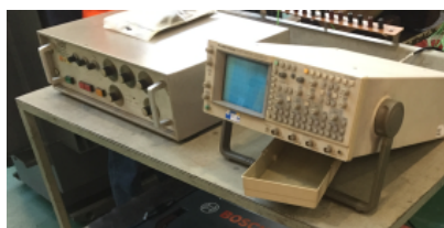
Fig. 4. Recurrent surge generator and oscilloscope used on the experiments.
