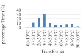
Solar inverter transformers operates in cyclic loading pattern in a 24 hour cycle. Also, their loading varies according to seasons & weather conditions. Loadings on solar inverter transformers are almost nil during night hours.
