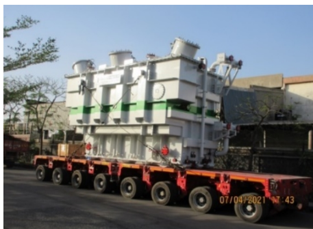
Reactor during transportation
