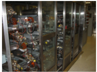
Example of dual temperature test cell that allows for independent control of conductor temperature and oil temperature. In the bottom, laboratory setup with dual temperature aging cells running.
