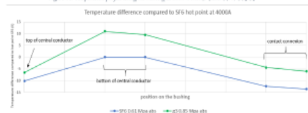
Figure 13. Temperature profile along the bushing at 4000 A with SF 6 and C 4 FN/CO 2
