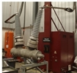
Figure 8: Picture of Dead Tank circuit breaker rated 143 kV under test.
