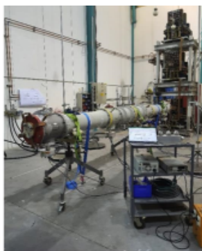
Figure 4: Picture of GIL under test
