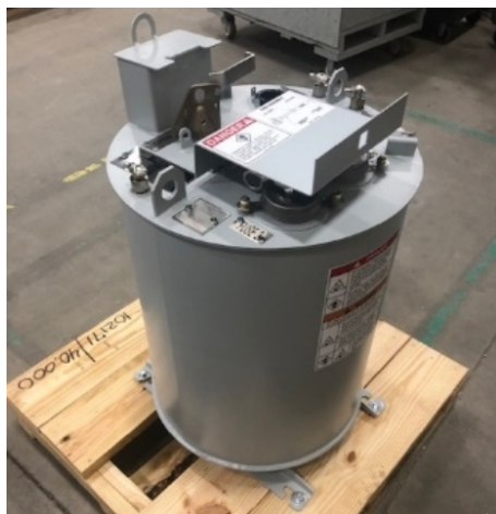
Rotary puffer (RP) in switch enclosure
