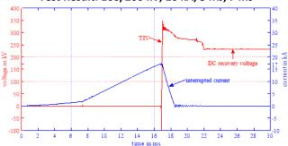
Test Result: 320 kV, 20kA, 10 MJ, 3 ms, 500 40 prospective cur 450 36 Transient Interruption Voltage (TIV 32 400 28 ≥ 300 ≣ 250 24⊴ DC recovery voltag 20년 16 12 12 250 200 200 200 200 nterrupted current 8 4 50 0 2 4 6 8 10 12 14 16 time in ms 18 20 22 24 26 28 30
