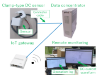
Fig.2 Overview of our monitoring system
