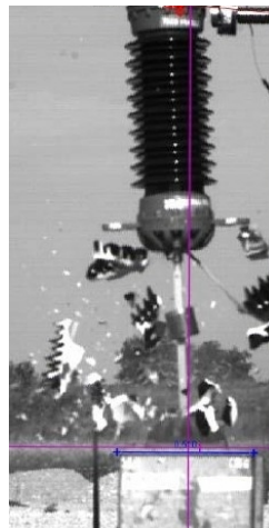
Rupture of insulator housing during a destructive mechanical stress test and projection of debris
