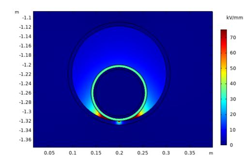
→ Unclear result due to high field concentration in the gap between cable sheath and plastic pipe.
