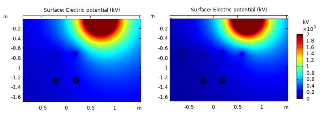
The picture shows the influence of 2 or 4 shield wires over a pair of HVDC cables.
