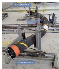
Tensile bend test on a 3-core power cable (Top), Strain vs cable length results (Left down), and 3-point bend testing on another 3-core power cable (Right down)
