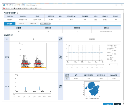
Figure 7. Result of PD analysis using AI algorithm in U-phases
