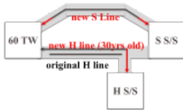
Fig. 5 H line replacement work utilizing S line
